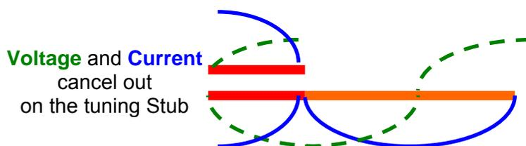
Again keeping it simple with voltage in Green and current in Blue, can you see how the voltage and current on the Stub cancel each other out ??? - leaving only the voltage and current of the half wave extension to do all the work and radiate a signal as seen below.
