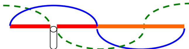
Can you see that the voltage and current distribution of the half wave extension is opposite that of the dipole ???
