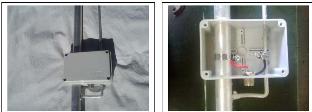
Inside the box I join the SO239 to the tube and stub - IT DOES NOT MATTER WHICH SIDE YOU CHOOSE to clamp the wires as it will work just the same either way. In the pictures above I clamp the Red to the tube and the Black to the stub. Don't let anyone tell you it matters which side it should go.
