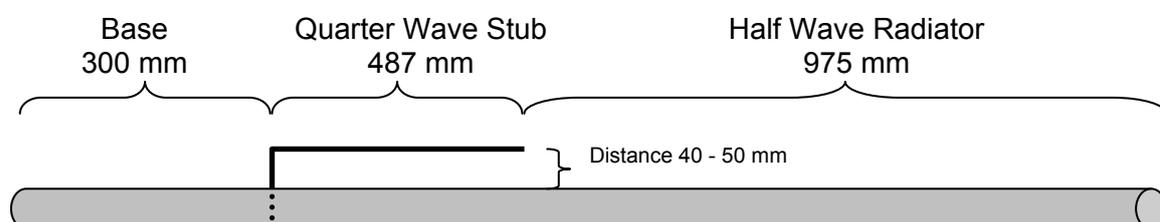
Leaving about 300 mm for the base allows the structural design to be extremely durable and sturdy. At my QTH my Zepp antenna has withstood every storm for the last 25 years - not many antennas can boast the same.
