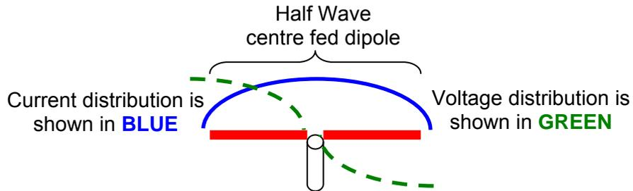
Now to explain the workings of a half wave Zepp or J-Pole I like to use a half wave dipole like the one below with one end of the dipole stretched and extended another half wave length until it looks like this.
