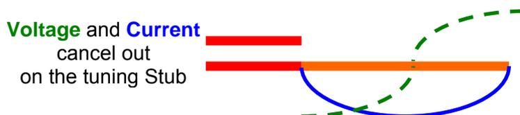
Engineers call an antenna that is feed this way a "voltage fed" antenna because the voltage is highest where the half wave extension meets the stub feed point. When it is stood up as a vertical it will radiate an omni directional pattern. When more "phased" extensions are added it will produce gain over a dipole with very pleasing reports.
